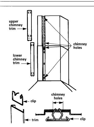
Cut upper chimney trim to correct length. Attach trim strips with clips to cover chimney seam.
